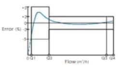
A. The maximum allowable error of a low area (Q1 ≤ Q < Q2) is ± 5%
