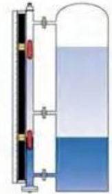
Style I Dual Indication for total interface level detection
